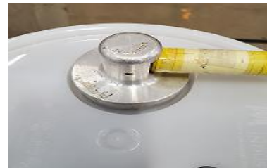
80 mm Screw Cap Tightened with torque wrench:
